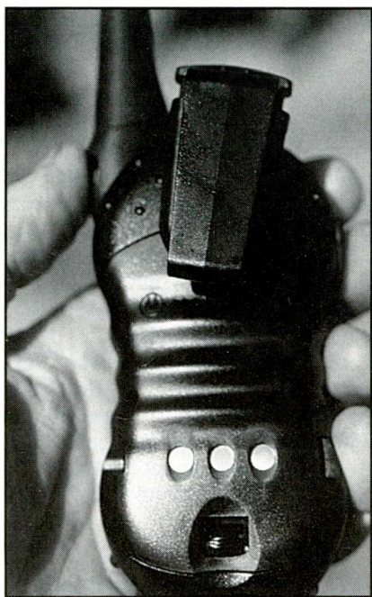
Motorola drop-in charger contacts.
